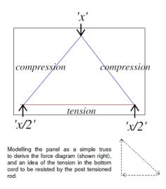
With no post-tensioning, the lower section of the panel cracked with a loading of 23.8kN. After post-tensioning with a force of 40kN applied to the bottom cord, the panel supported a load of 89.4kN, resisting a Bending Moment of 50kNm.
